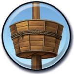
A crow's nest is a structure in the upper part of the mainmast of a ship, that's used as a lookout point. In early ships it was simply a barrel or basket lashed to the tallest mast. Imagine that?!
