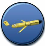
The Slocum Glider, used by the Mote Marine Laboratory, is an amazing tool that collects data from our ocean waterways. These sleek rocket-shaped machines gather important scientific information, and transmit the findings back to base through a satellite system. What a clever devise, aye?!
